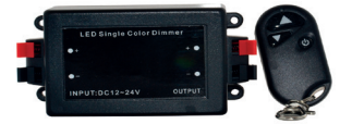
R004 Wireless dimmer 12V/24V with Remote- 5M. Max 6Amp L115 x W56 x H34 Max wattage: 12V:96W 24V:192W
