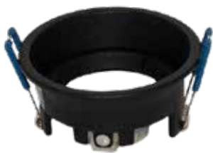
R218 BA919 Slim Anti Glare • Black CNC Aluminium Ø80 x H37 / Cut 69 - 72
